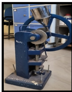
Fig. 1: Tablet compression machine used for the preparation of core tablets by direct compression method.
