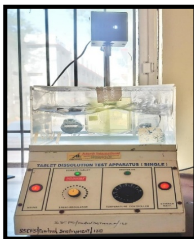
Fig. 13: USP Apparatus II (Paddle method) used for In-vitro dissolution study.
