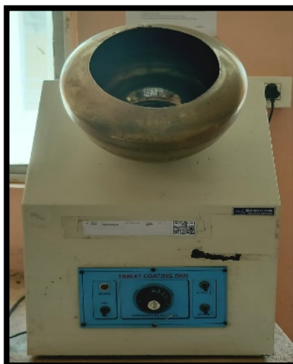
Fig. 2: Laboratory-scale pan coating apparatus used for manual spray coating of tablets.
