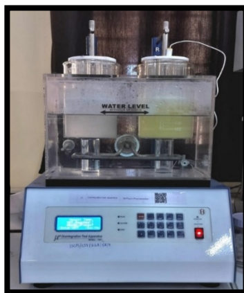
Fig. 11: Disintegration test apparatus showing the disintegration behavior of film-coated pulsatile Epalrestat tablets in distilled water maintained at 37 \pm 0.5^\circ\text{C}
